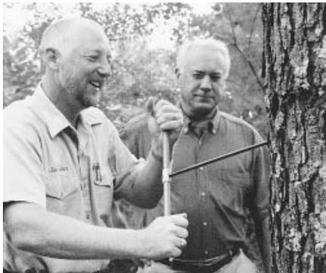
Jim Jeter, forest management specialist for the Northwest Region, demonstrates an increment borer for a landowner.
