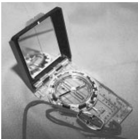
A good quality cruiser's compass is a standard tool for forest owners.
