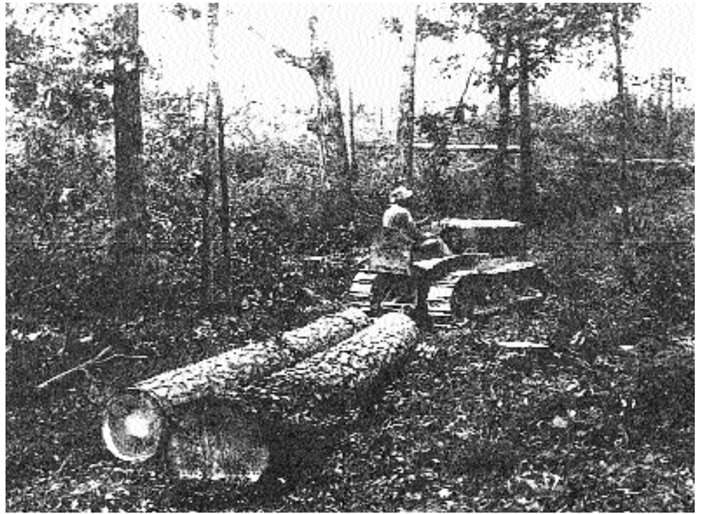
There's no winch, only a chain wrapped around the back of this Caterpillar crawler-tractor, on U.S. Steel land in Jefferson County in the 1940s.
