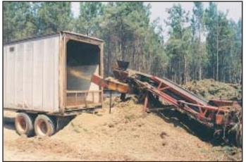
Finer chips made from tops and limbs are blown from the grinder into a large enclosed truck for transport to a boiler or storage facility. *Fall 2004*
